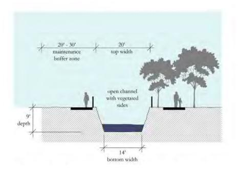
Minimum engineering requirements for an open channel. A naturalistic alternative is possible with additional land area.
